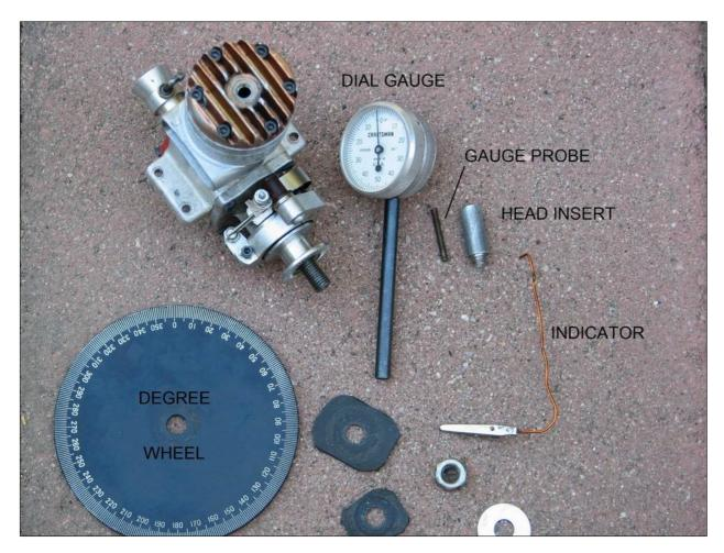
Well, actually it shows a bit more than what's really needed. The machinists dial gauge gives a more accurate reading of the pistons top dead center (TDC) location, but isn't strictly necessary. The gauge probe and head insert had to be custom made to use the dial gauge. The head insert screws into the spark plug hole. It's hollow to allow the longer than stock gauge probe to reach in and touch the piston top. I made an insert for each of the two plug sizes.
