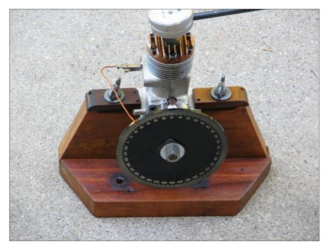
This view shows the indicator wire in place, along with the dial gauge for establishing TDC. The dial gauge isn't locked in, but is just hand held solidly in place while rotating the wheel and taking readings.
