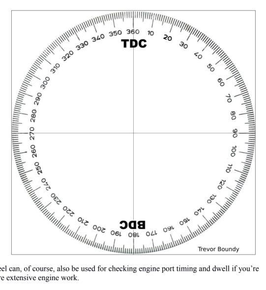
The wheel can, of course, also be used for checking engine port timing and dwell if you're into more extensive engine work.
